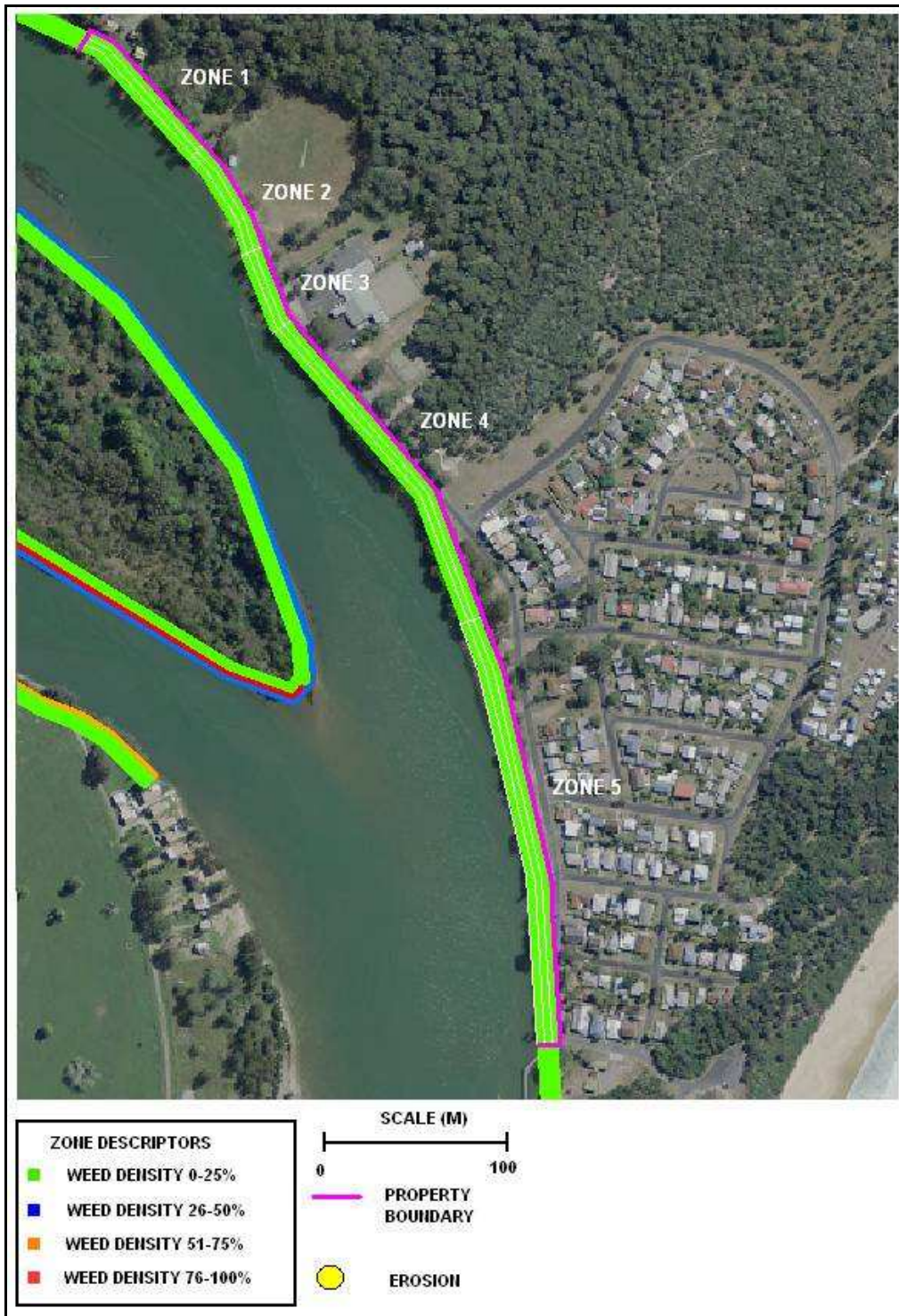
Figure 128: Riparian condition and extent
