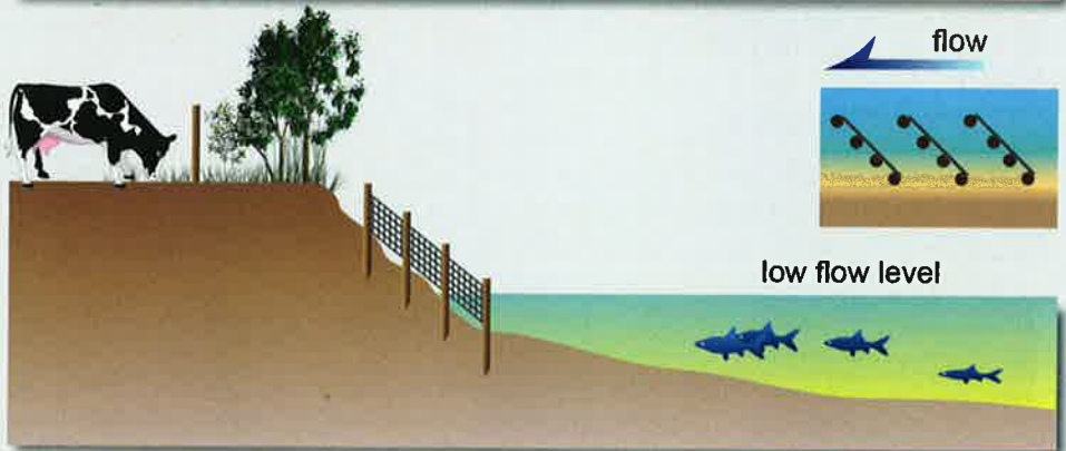
Mesh Pin groynes
